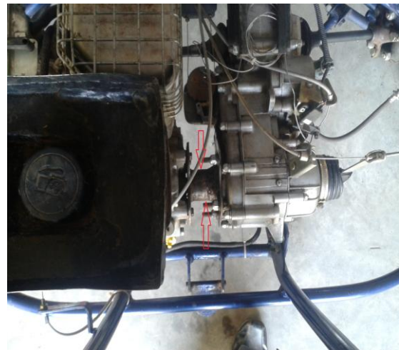
Figure 6. Adapter shaft installed in the vehicle
